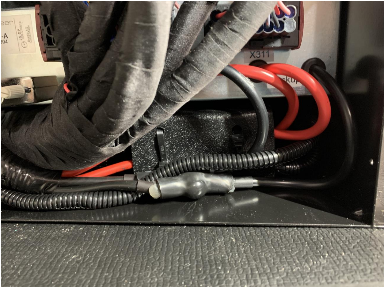
This picture shows the Egress Relay with its insulation to prevent any shortcuts
