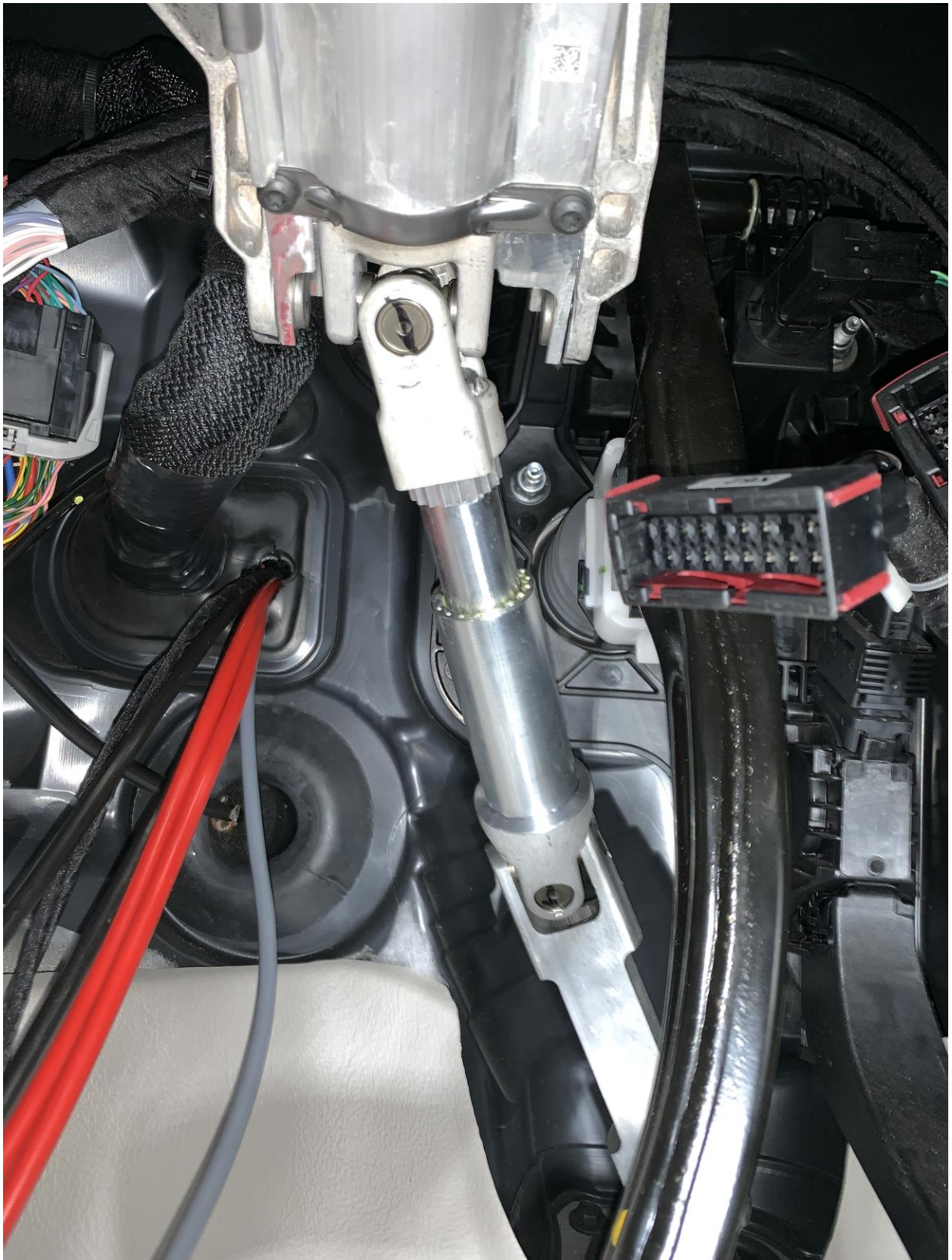
Picture shows the battery cables coming from the engine compartment. An original opening can be used. No need to open the firewall.
