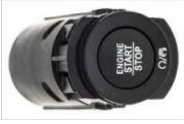
IDENTIFYING THE ENGIN START STOP SWITCH (ON RIGHT SIDE OF STEERING)
