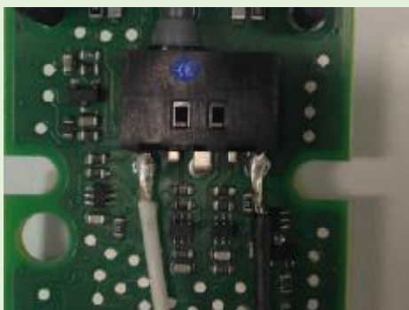
Example of soldering two wires on the internal switch
