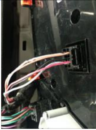
IDENTIFYING THE HAZARD SWITCH LOCATION, AC MODULE (ON CENTER CONSOLE)
